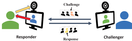
Fig. 2. Challenge-response process of LiveScreen leveraging the inconspicuous light reflected off the human face for video liveness detection.
