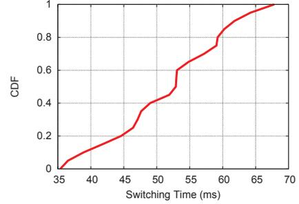
Fig. 2. CDF of switching time for *CogFrame* when using a Wi-Fi RF-frontend.
