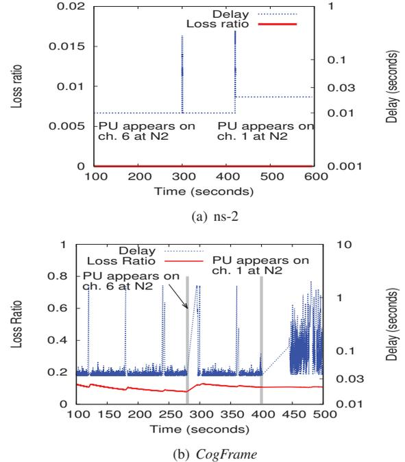
Fig. 4. The performance of LAUNCH on ns-2 and *CogFrame* in terms of delay (log-scale) and loss ratio.
