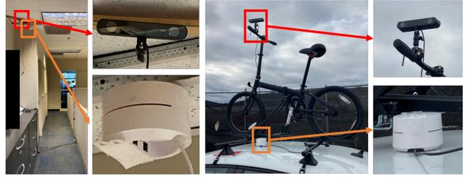
Fig. 4. Experiment Setup. A StereoLabs ZED2 camera and a Google Nest WiFi AP mounted on the ceiling in the *Indoor* setup while the camera is mounted on the handle of a roof-mounted bike for outdoor setup. This setup simulates increasingly common WiFi-enabled cameras.
