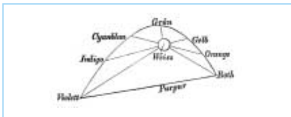
Figure 1.18 The first chromaticity diagram to have a modern form, prepared by Helmholtz on the basis of his measurements of complementaries.
