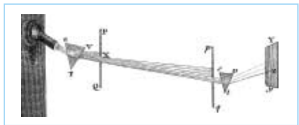
Figure 1.1 An eighteenth-century representation of Newton's Experimentum crucis . As the left-hand prism is rotated around its long axis, the beam selected by the two diaphragms is constant in its angle of incidence at the second prism. Yet the beam is refracted to different degrees at the second prism according to the degree to which it is refracted at the first. (From Nolle's Leçons de Physique Expérimentale ).
