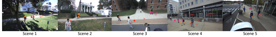
Figure 5: Showcasing localization results for five test scenes. Each user’s estimated 3D coordinates with respect to the RSU’s camera are projected into the image and highlighted by different markers of the same color. The solid squares represent the ground truth location of the users; the hollow squares represent raw GPS measurements; the hollow circles represent the FTM-fused GPS locations; the solid circles represent our GAN-generated location estimations. Our method’s estimated locations are the closest to the ground truth (Best viewed zoomed).
