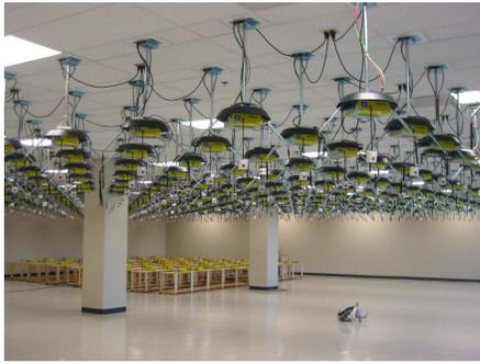
Fig. 1. ORBIT Testbed setup consisting of 400 small form-factor PCs with two 802.11 wireless NICs each.
