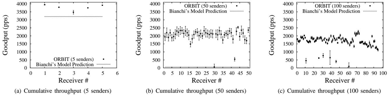
Fig. 2. Empirical mean and std. dev. in cumulative throughput (packets per sec.) at each receiver. Note that empirical throughput is much higher than what Bianchi’s model predicts. In the case with 100 senders, the model predicts a throughput of 2 pps (not visible).
