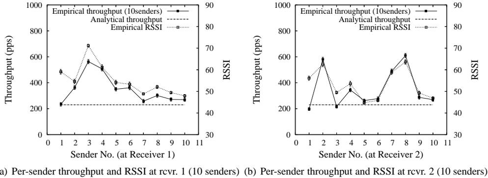
Fig. 3. Empirical mean and std. dev. in per-sender throughput and RSSI at 2 receivers in the 10 sender, 10 receiver experiments. Note that there is good correlation between per-sender throughput and RSSI.
