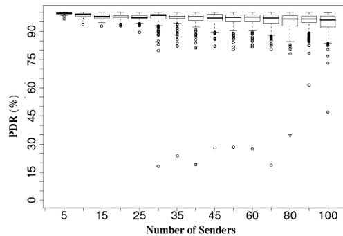
Fig. 4. Boxplot (five-number summary) of PDR for varying vehicular densities. Note that the boxplot is calculated over different time intervals and across different receivers.
