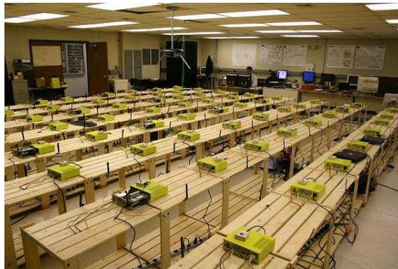
Figure 1: *The ORBIT indoor testbed, comprising of 128 IEEE 802.11 a/b/g interfaces, attached to 64 stationary nodes, arranged in an 8 by 8 grid*
