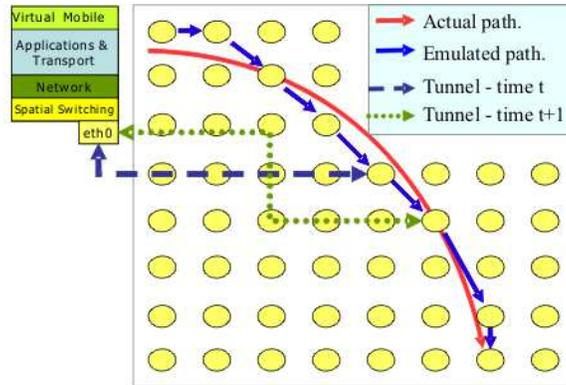
Figure 2: *Mobility emulation through spatial switching. All layers above the MAC reside on the “Virtual mobile” node, throughout the experiment. The link and physical layers of different nodes on the grid are used over time, based on the specified mobility pattern.*
