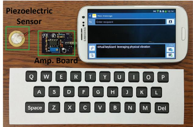
Figure 1: The *VibKeyboard* platform prototype.
