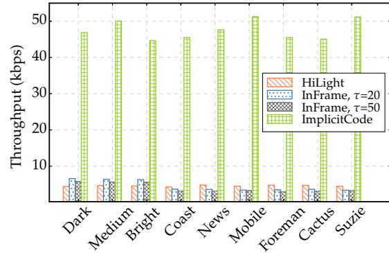
Figure 12: Measured goodput of ImplicitCode vs HiLight and InFrame.
