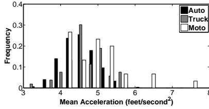
Figure 2: Histogram of mean acceleration for trucks, autos and motos.
