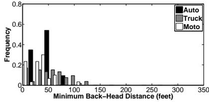
Figure 6: Histogram of minimum back-headway distance for trucks, autos and motos.
