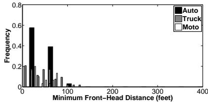
Figure 7: Histogram of minimum front-headway distance for trucks, autos and motos.
