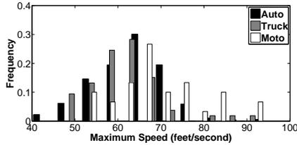
Figure 3: Histogram of maximum speed for trucks, autos and motos.
