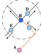
Fig. 1. An example handoff situation. In this case,  $B$  is the initial carrier. MPF will choose node  $E$  as the relay (because its distance with  $A$ , the anchor location, is decreasing and it is currently the closest to  $A$  among all the nodes), while trajectory-based schemes will choose  $C$  as the relay.
