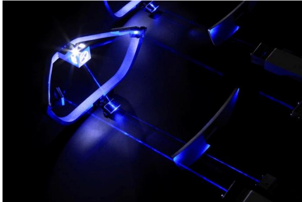
Figure 1a – Three blue lasers reflect off planar mirrors and hit a yellow phosphor to produce white light.
