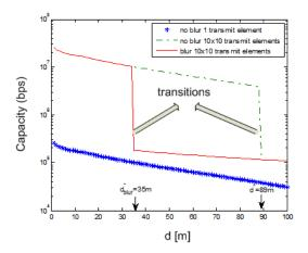
Fig. 5. Visual MIMO channel Capacity versus distance ( $\phi = 0$ )
