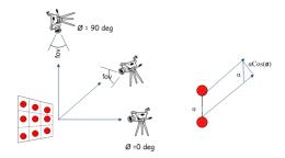
Fig. 3. Camera Viewing angle Illustration
