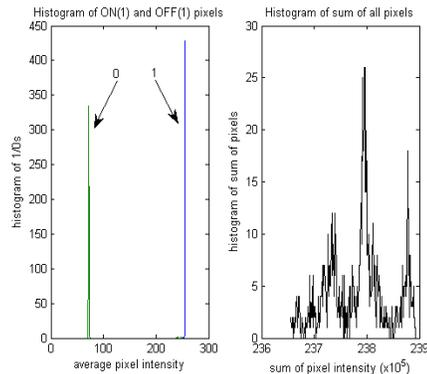
**Figure 3: Histogram plots of Basler Pilot piA640 camera snapshots in medium sunlight(left: $10 \times 10$ , right: $640 \times 480$ )**
