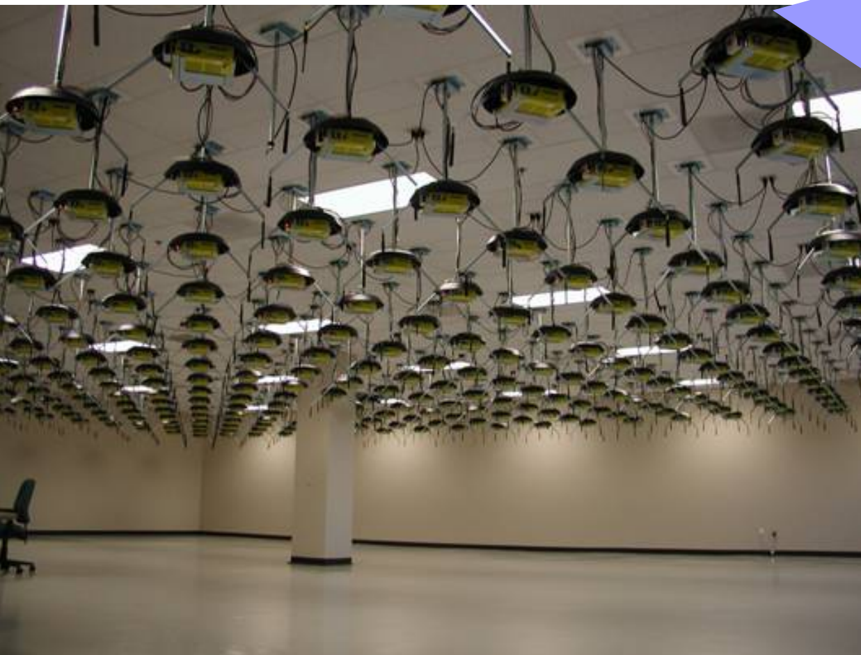
400 Node High-Density Controlled Indoor Testbed
