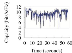
(b) A leaky-feeder cable at walking speed.
