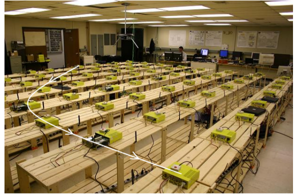
Figure 1: Spatial Switching. The path shows an actual path of a mobile node, which the system emulates by choosing the radio node that best approximates the current position. The testbed comprises currently 64 nodes with two 802.11 a/b/g interfaces each.
