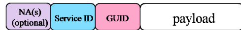
Fig. 3: Chunk ‘packet’ with key fields. While GUID is the authoritative routing information, the NA (if bound) provides fast forwarding path.
